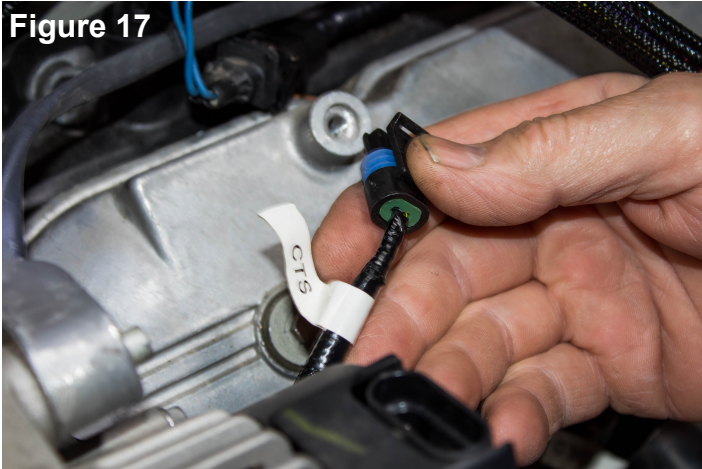
Above - Our CTS plug is made to work with the factory OEM temperature sensor. Replacements are also available if needed.
